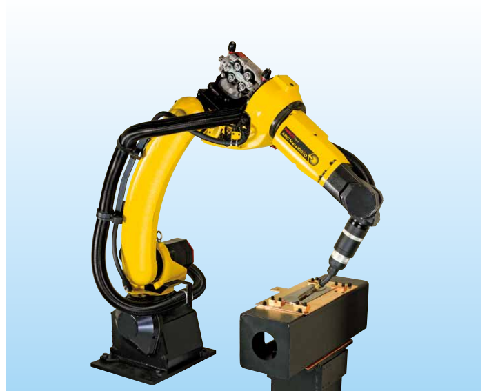
Stainless part welding
